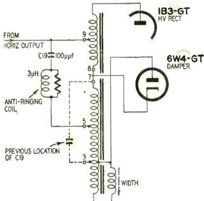
Fig. 2—Flyback circuit in the Pacific Mercury 150.
