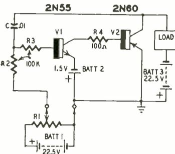
As C charges, Junction C-R2-R3 goes less negative. When the base voltage has dropped to about 1.5, V1 begins to conduct. Current flows through R4 to unblock V2 as well. C now discharges through R3 and saturates V1, and in turn V2. Thus, a second discharge path exists through R2 and V2.
