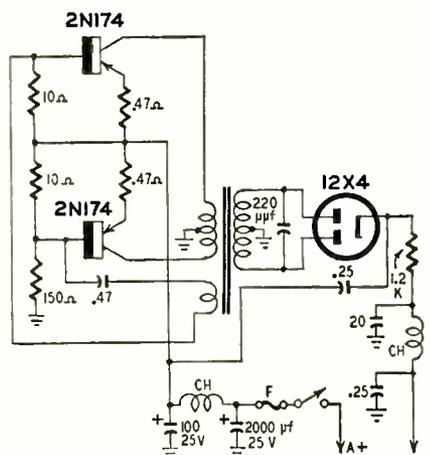
Fig. 10—Transistorized power supply replaces familiar vibrator.
