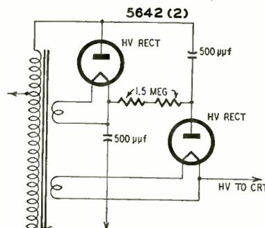
Fig. 1—The 500- $\mu$ f capacitor measured 700,000 ohms. It caused blooming by lowering the high-voltage output.
