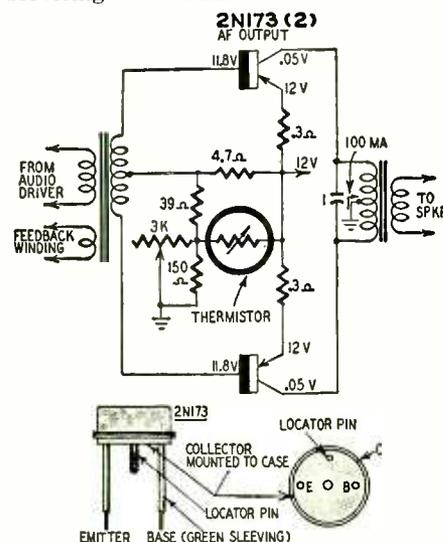
Fig. 12—Delco output stages use thermistor to protect transistors against overheating.
