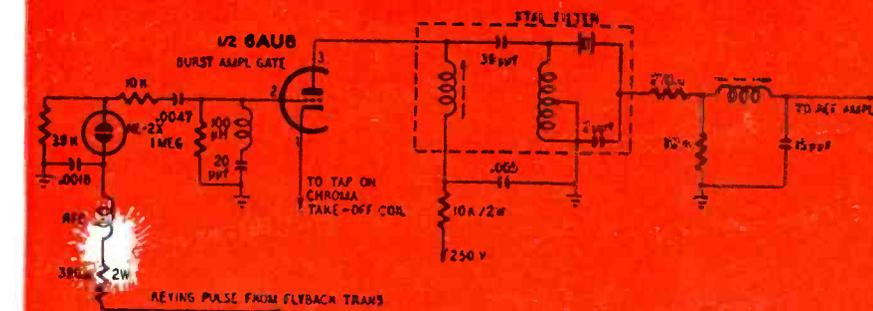
Fig. 1—Neon lamp in color-burst keyer maintains keyer-pulse amplitude constant
