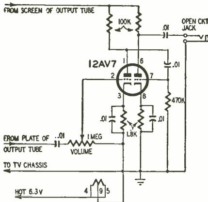
2—100,000-ohm 1/2-watt resistors; 1—470,000-ohm 1/2-watt resistor; 2—1,800-ohm 1-watt resistors; 1—meg-ohm potentiometer; 5—.01- $\mu$ f disc ceramics or tubular capacitors; 1—12AV7 tube; 1—9-pin miniature socket; 1—open circuit jack; 1—chassis.
