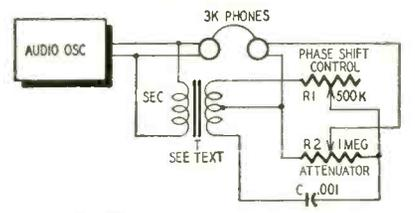
A suitable demonstration arrangement is shown in the diagram. T is a conventional audio output transformer with its low-impedance winding connected to the audio oscillator. R2 operates as an ATTENUATOR and should be set to provide approximately the same level of sound in the right earphone as in the left. R1 is the PHASE-SHIFT CONTROL, and causes the apparent direction of sound origin to move around the listener as its setting is varied.—Robert G. Middleton END
