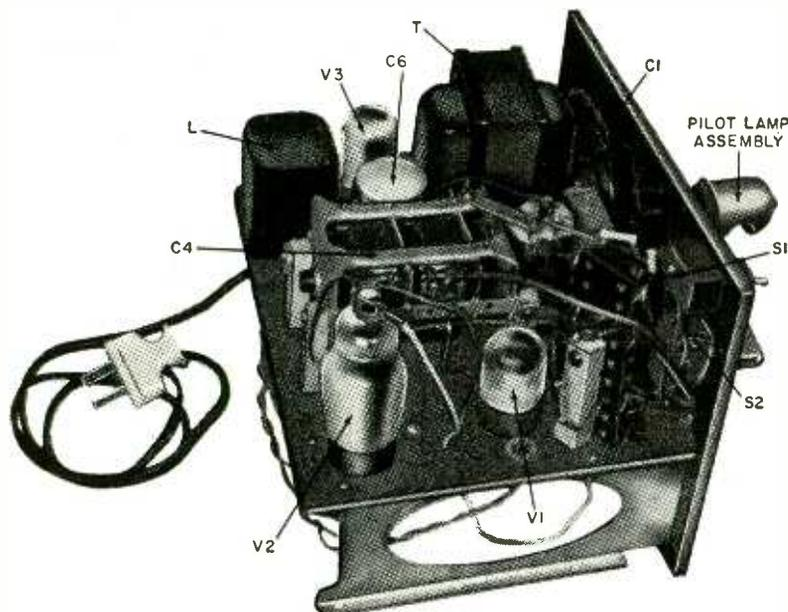
Internal view showing layout of important components.
