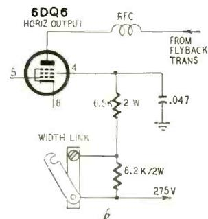
This circuit (*b*) supplies approximately the same screen voltage but puts the .047-μf capacitor directly between screen and ground, effectively removing the isolating or screen suppressor resistor and reducing the width. Replace the single resistor with the two proper values. The 6DQ6 socket has two spare pins which can be used as tie points.—
