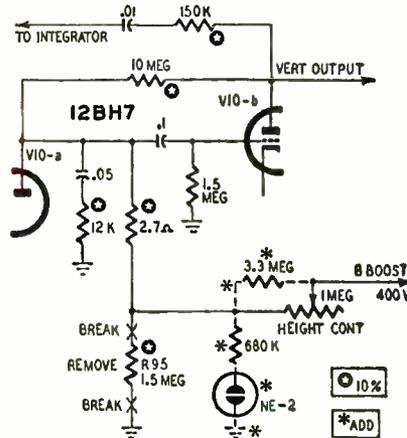
Fig. 4—Bypass action is combined with primary voltage-regulator action in this Olympic C21BD35 modification.
