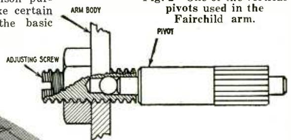
Fig. 2—One of the vertical pivots used in the Fairchild arm.
