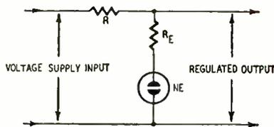
Fig. 3—Typical neon voltage-regulator circuit.
