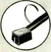
**Model 194D UNIPOISE Pickup Arm**—This new lightweight . . . integrated arm and cartridge assembly containing the FLUXVALVE with exclusive "T-Guard" stylus—is only a fraction of the weight of conventional tone arms. High compliance and single friction-free pivot bearing assure distortionless tracking of microgroove and standard groove recordings. Available with the 1/2, 1 or 2.7 mil diamond stylus. Prices from \$59.85.
