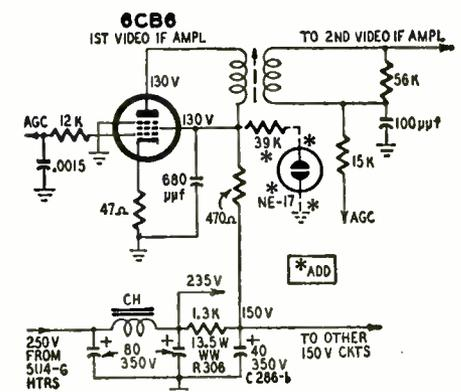
Fig. 6—Neon bulb as a glow-lamp regulator cured a case of jitter in this Dumont RA-350.
