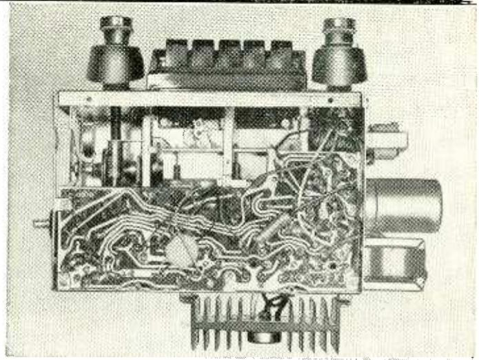
radio's volume as the speed of the engine increases. With an increase in speed, wind and road noises get louder and the volume of the radio is automatically increased to compensate for this.
