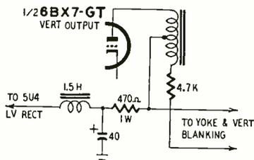
Fig. 2—Defective electrolytic passed dc ripple; picture rolled.
