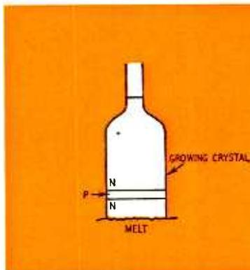
Fig. 2—A grown n-p-n sandwich suitable for transistors.
