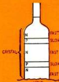
Fig. 3—Many junctions can be rate-grown in one crystal.
