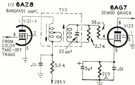
reveal low plate and screen voltage at V121-b, the bandpass amplifier. A positive voltage is found at the grid of V123, a demodulator driver. Turns out that T113, the bandpass transformer develops a high-resistance short between its primary and secondary—usually more than 1 megohm. Replacing the transformer is the only cure, and a quick one.—*Joe Shane*
