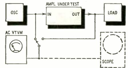
Fig. 5—Block diagram of a basic frequency response and output power test setup.
