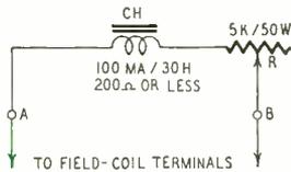
Connect a 5,000-ohm variable resistor (R) in series with a filter choke (CH) across the field-coil terminals. Vary R until proper plate and screen voltages appear. Then turn the power off and measure the resistance between points A and B. Now just hook up a coil with the same value.—Stanley Clark
