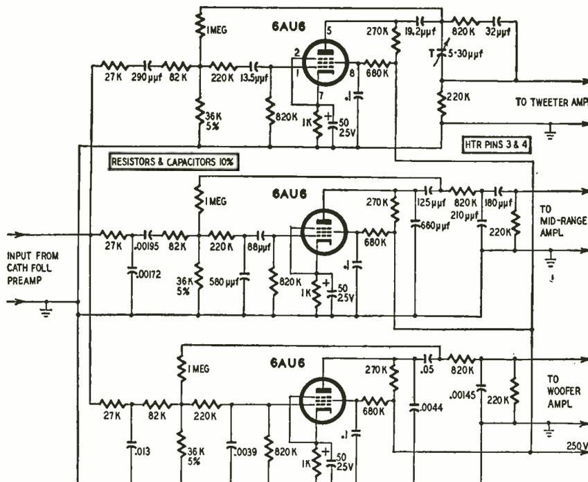
NOTE: When purchasing parts for this circuit, use parts list for Fig. 5 and multiply the number of individual components by the number of channels in the system. Some capacitors are omitted in the tweeter and woofer channels. See text.
