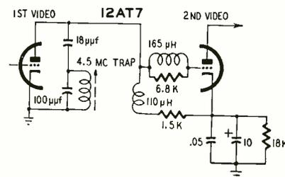
Fig. 3—Low resistance short in the .05- $\mu\text{f}$  capacitor lowered plate voltage and caused lack of contrast.
