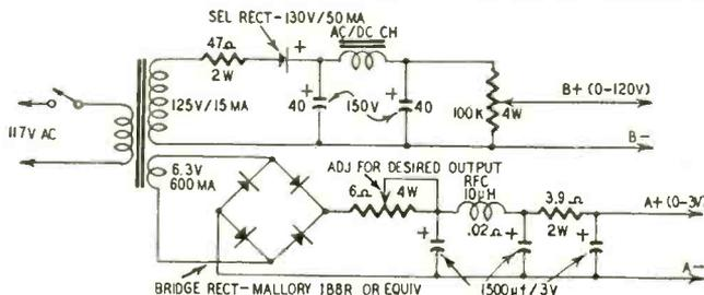
The circuit of a suitable eliminator is shown in the diagram. It can be used with most portables with parallel-connected 1.5-volt filaments. B voltage can be as high as about 120 with normal drain and A voltage can be adjusted to supply some sets requiring 3 volts. The eliminator can be improved by installing a 25-ma dc meter in the
