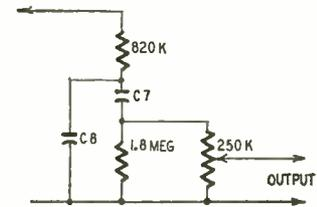
Fig. 8—How to combine the amplifier's gain control with outputs of Fig. 6 to provide a balance adjustment.
