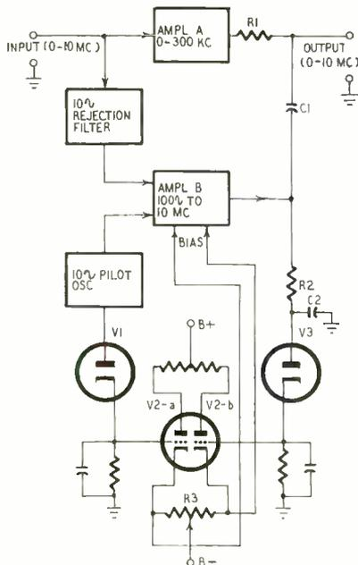
There must be no coupling between A and the pilot generator. Also, the pilot frequency must not reach B directly from the input. Both purposes are accomplished by a rejection filter.
