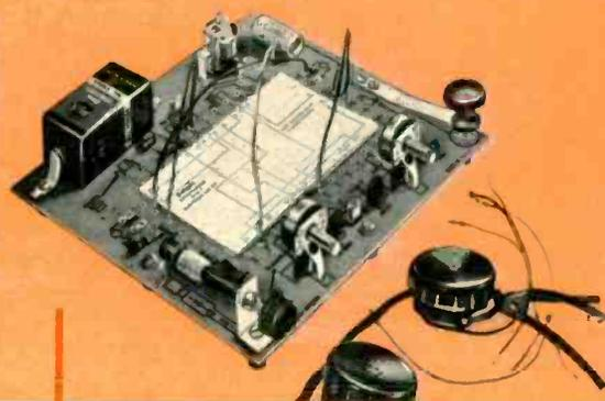
**knight-kit 2-Transistor Pocket Radio Receiver Kit**
