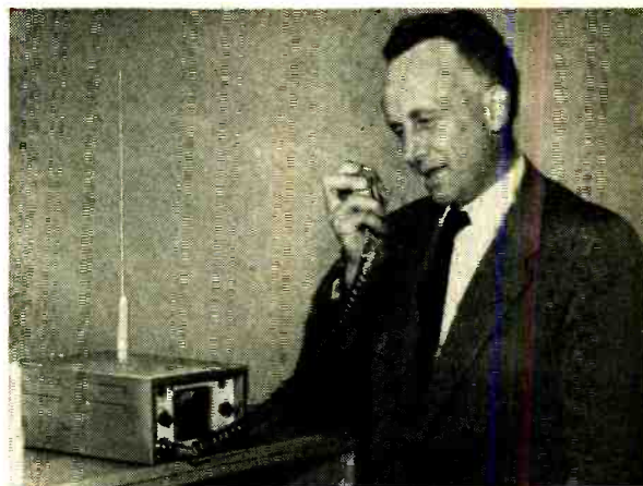
Low-power industrial or Citizens band radiotelephones can be used for private ship-to-shore communications.
