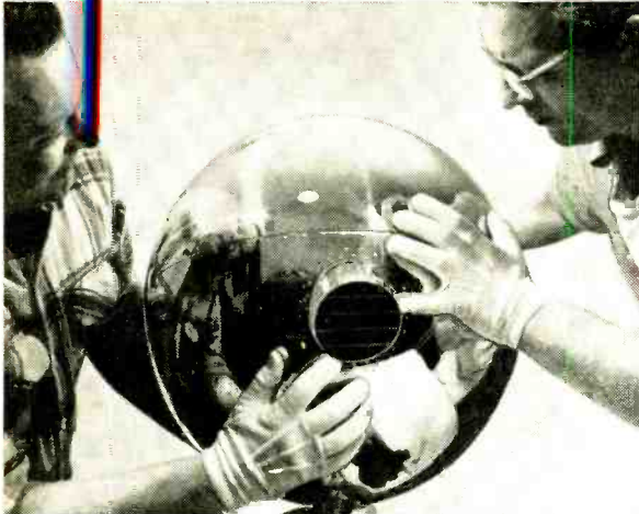
Ready to launch, the polished satellite is handled with soft gloves to avoid marring its finish.
