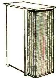
STEREOFLEX II: Double horn-loaded, using an extended air column mid-range with heavy duty compression driver and 3000 cps crossover wide-angle tweeter. Built-in BRILLIANCE control. Response: 150 cps to beyond audibility. Hardwood furniture finishes. 25 1/2" h. x 10" w. x 19 1/2" d. User net: Mahogany—$110.00, Blond or Walnut—$113.00.
