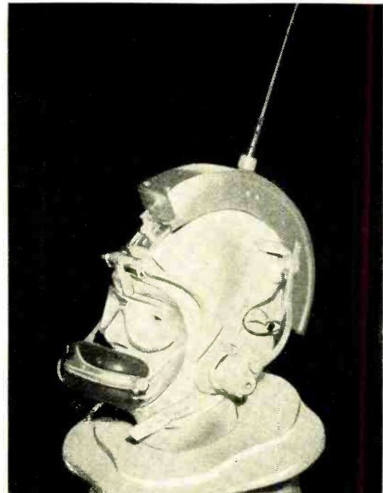
Helmet transceiver developed for carrier jet-landing instructions by Dr. Webster and Mr. Gibson of the Naval Electronics Laboratory in San Diego, Calif.
