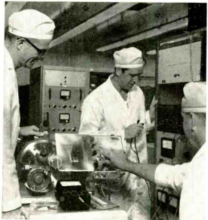
Inertial guidance gyros, accelerometers and other critical components are assembled, inspected and tested in air-conditioned dust-free rooms to prevent contamination and resultant inaccuracies.
