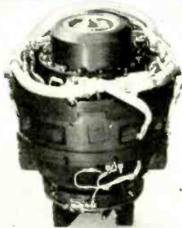
Gyroscope used in 5,000-mile range missiles has extremely low drift rate.
