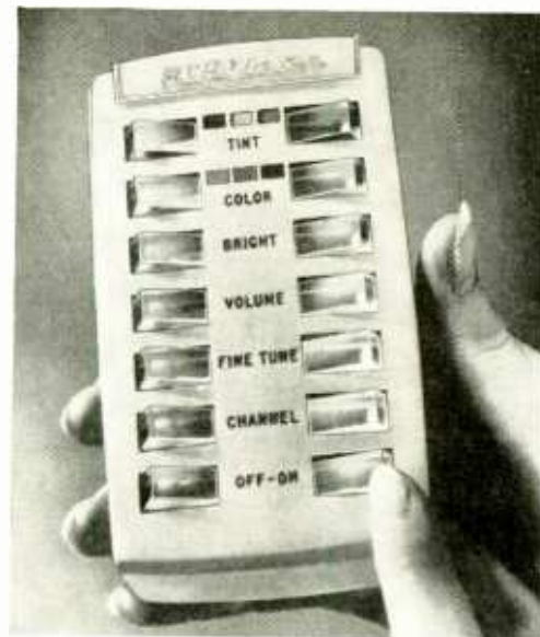
Transistor-powered Wireless Wizard for color TV provides remote adjustment of color receiver controls.
