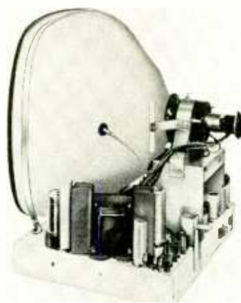
Zenith chassis uses a finned power transformer.
