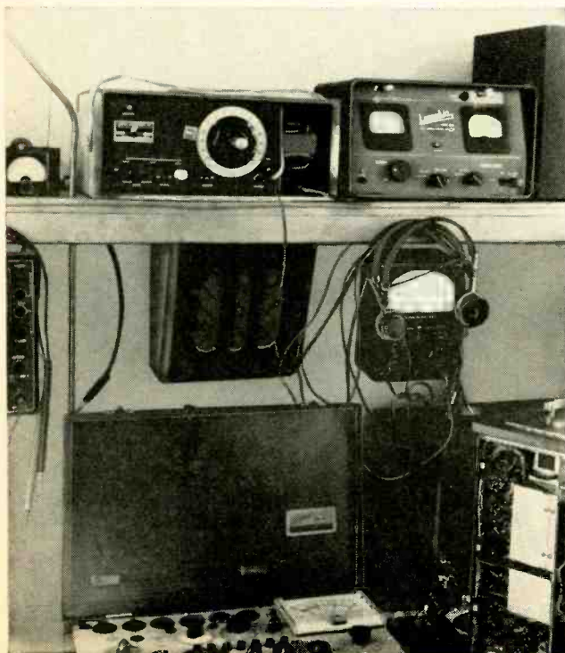
Essential instruments for servicing 2-way radio. On the shelf at the far left is a relative field-strength meter. In the center is a frequency meter for measuring transmitter frequencies. It can also be used as an rf signal generator. At the right is an FM deviation meter for measuring transmitter modulation. The vom is obvious and the tube checker is a mutual-conductance type.
