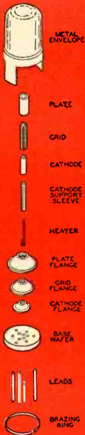
Fig. 1—Exploded view of the nuvistor triode.
