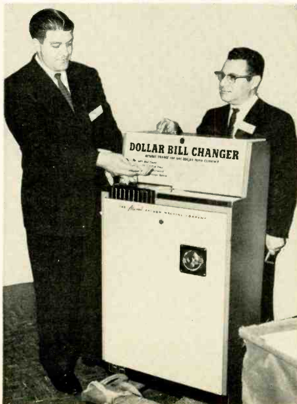
Simply insert a dollar bill in the rack on top, push it into the machine, and the change is returned in the cup below.
