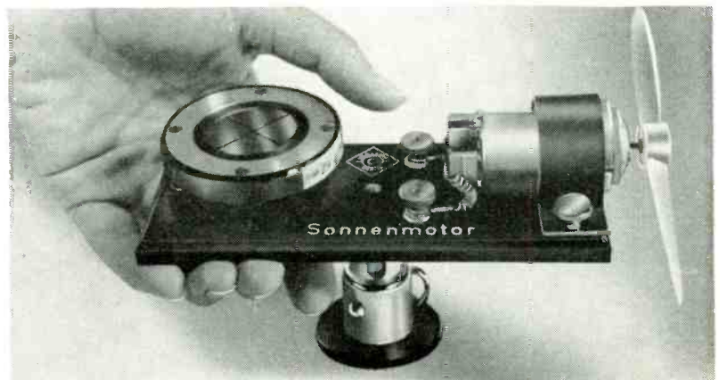
SUNMOTOR (2 volts at 200 ma) drives fan from silicon photocell. The little device was constructed by Dr. Bruno Lange of Berlin on his 25th anniversary as a photoelectric cell manufacturer. The motor runs even on light from ordinary household bulbs. Efficiency is about 10%.
