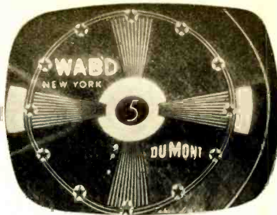
Left-hand foldover caused by excessive plate voltage on the horizontal oscillator in a Synchroguide sweep system.
