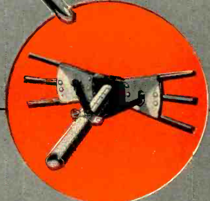
Calibrated sleeve for quick peaking of antenna.
