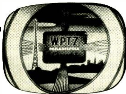
Fig. 1—Antenna is misoriented by 90°.
