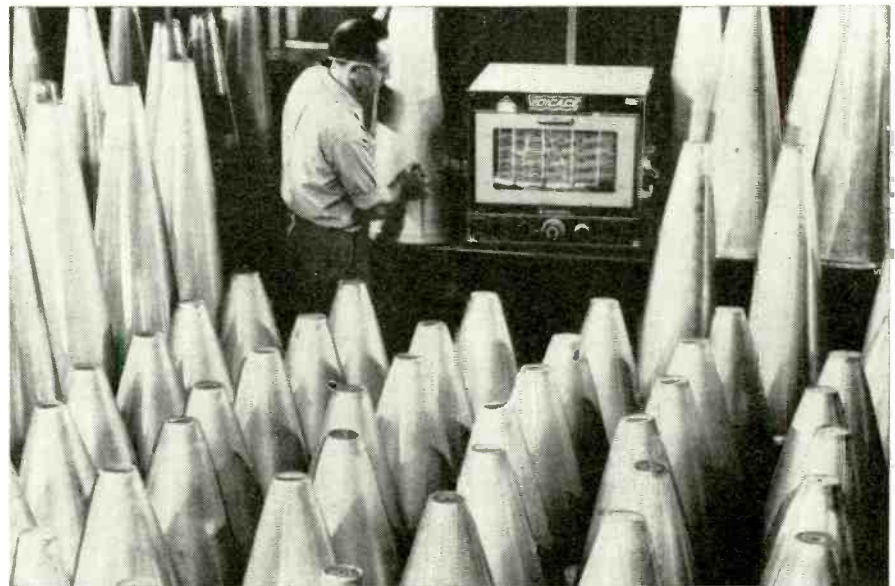
Ultrasonic gauge tests thickness of nose cones for Nike-Hercules missiles.
