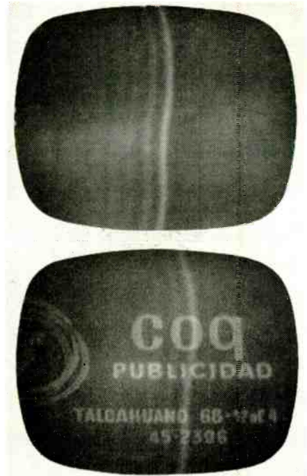
Halos caused by the porch level appearing during retrace.
