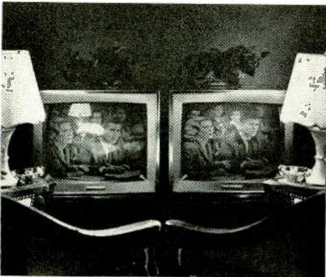
Two TV sets that are identical in all but the picture tube show the effectiveness of the reflection-free tube face introduced by the Corning Glass Works. Corning's new tube is on the right.
