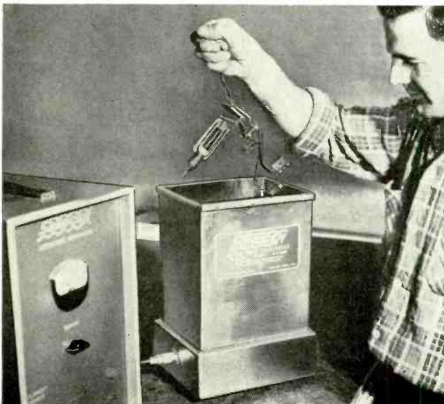
Ultrasonic setup for cleaning miscellaneous metal parts.
