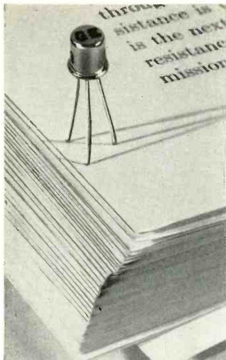
G-E's gallium arsenide tunnel diodes measure only a fraction of an inch in any direction.
