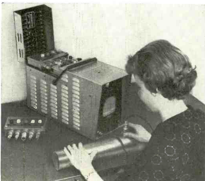
Ultrasonic flaw detection in machine stock. Indentation in scope baseline indicates a flaw.
