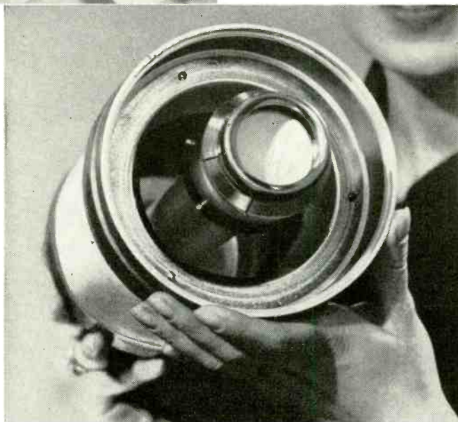
Super-power electron gun. Intensity of electron beam is equivalent to concentration of 5 million 40-watt light bulbs.
