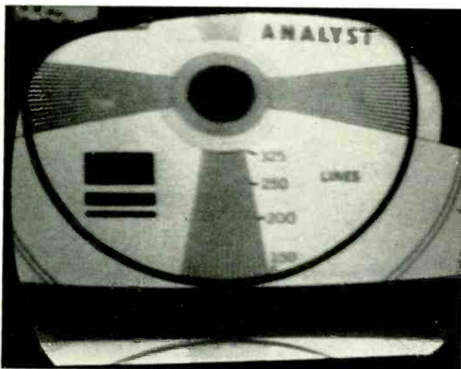
Feeding sync pulses to the grid instead of the plate (Fig. 10) locked in the picture with the blanking bar visible.
