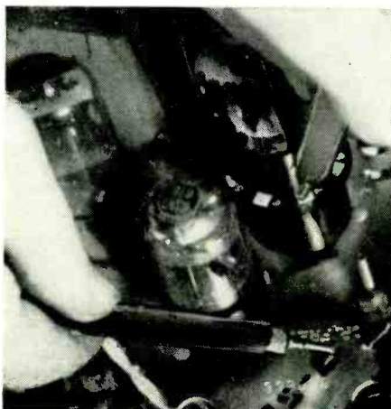
Checking tube-element voltages from the top of the chassis. All it takes is a test-socket adapter.
