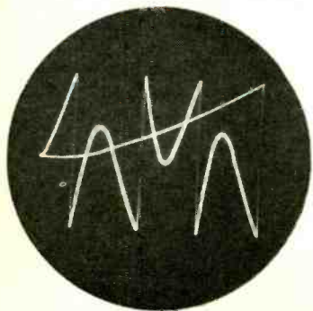
Fig. 10—Combination sine and square waveform.
