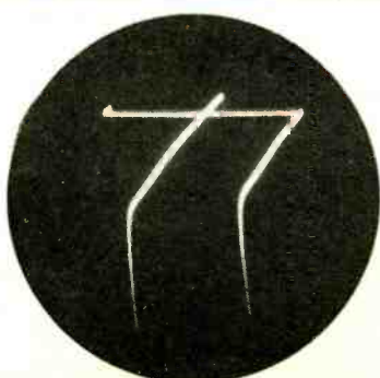
Fig. 11—Combination of a pulse and a sawtooth.
