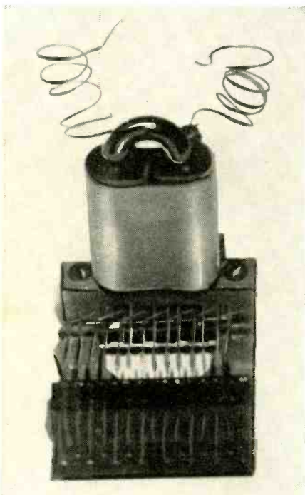
Delicate silver wire contacts of pipe-organ relay do not carry much current. Since many of these units are used in a single organ, they must be inexpensive.
