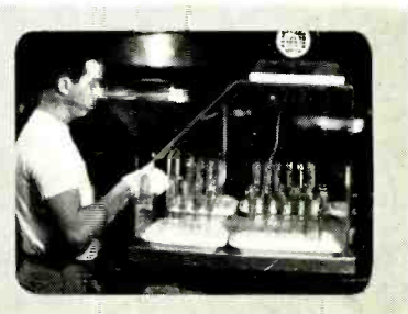
Guns await final assembly in this pressurized plastic housing. Blower at top maintains pressure, prevents dust from entering housing.
