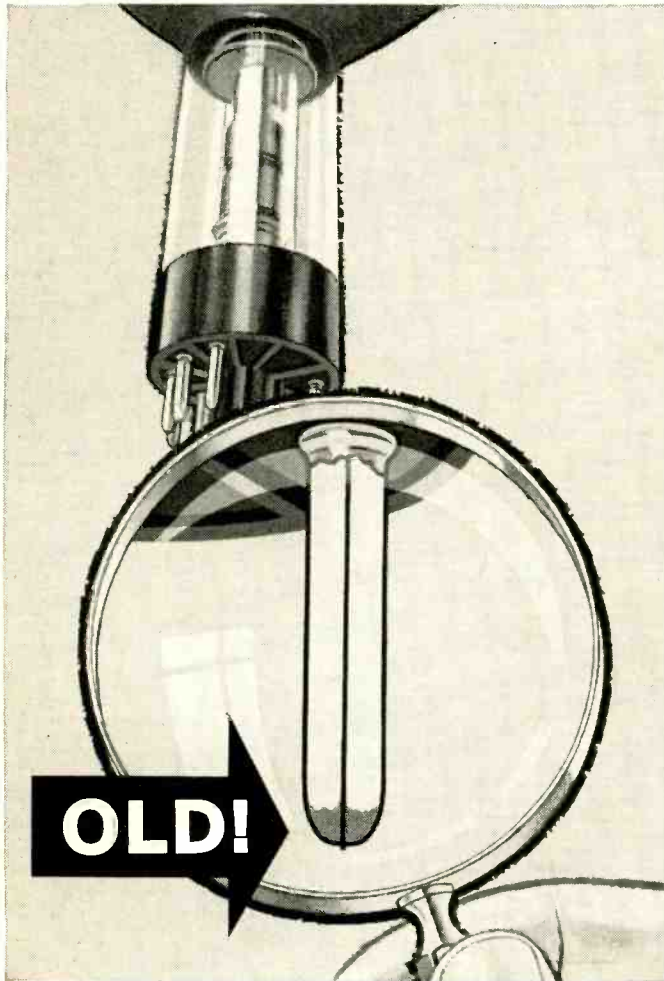
The "old" conventional pin soldering method relied upon contact between pin and wire only at their tips.
