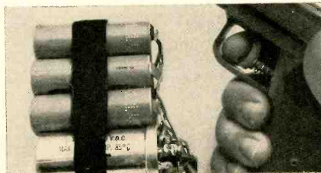
Pistol power supply is external. It is made up of 3 mercury batteries and a high-value electrolytic capacitor.
