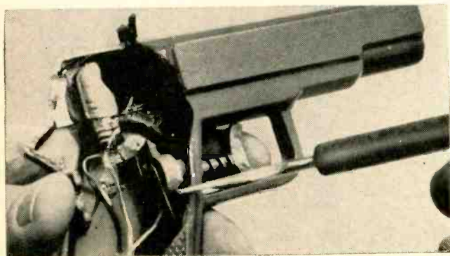
The electrical assembly mounted in the pistol.
