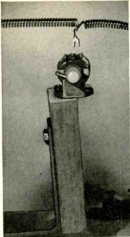
How the spring is attached to a ceramic cartridge. Damper block is also shown.
