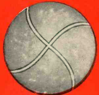
Fig. 7—The completely activated cathode.
