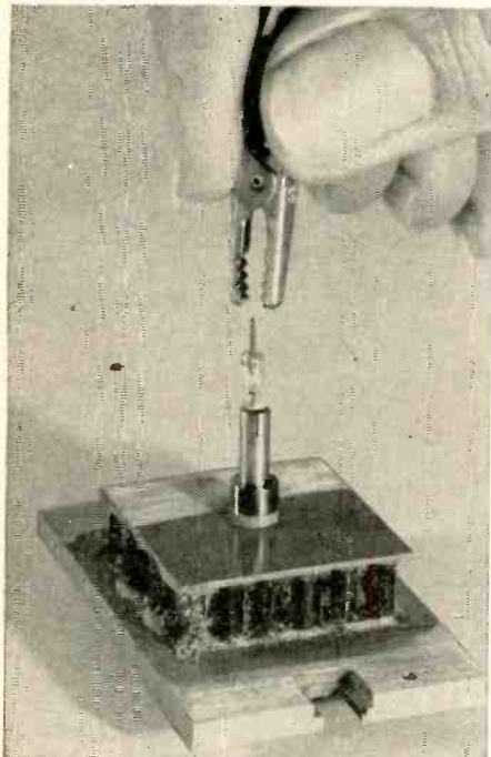
Experimental diode cooler for spot-cooling tests on electronic components.
