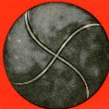
Fig. 6—More uniform diffusion as barium comes to cathode surface.
