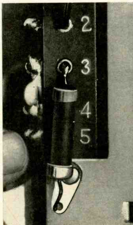
Philco's varistor is located just inside the high-voltage cage.
