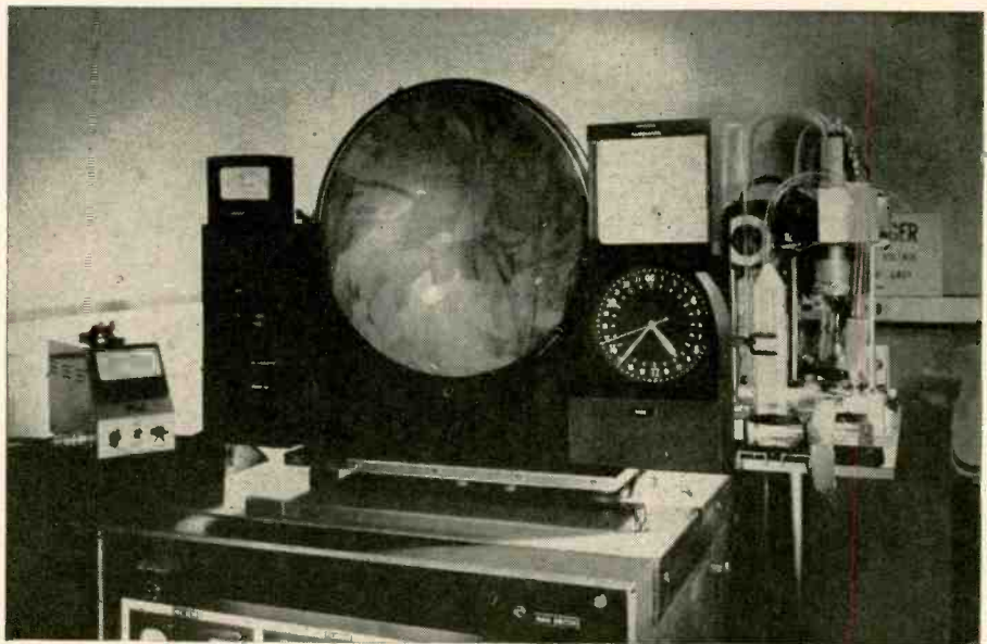
The pattern on the tube face can be photographed together with other instruments showing the time, pertinent voltages and other information, for a permanent record.
