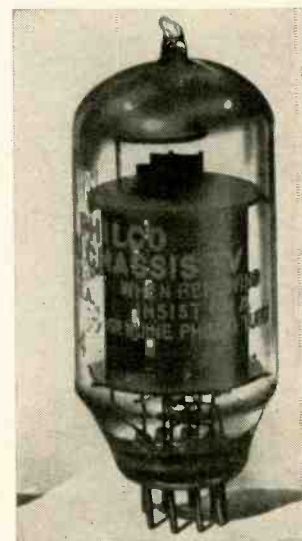
Philco's 6FD7 vertical output tube has standard 9-pin base and dissipates more heat by using a larger than normal glass envelope and heavier construction.
