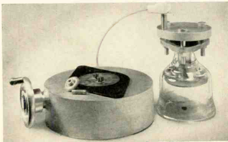
A prototype unit. The disc cathode can be seen in a bell-jar at right. The mask and a sputtered resistor are lying on top of the base. In the actual machine, the hand-wheel at left is replaced by a rubber-tire wheel, which rolls along a track to rotate the resistor and mask while being sputtered.
