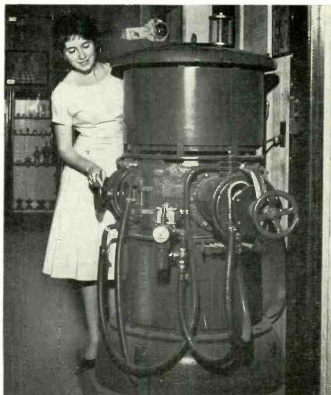
POULSEN ARC made daylight communications between the West Coast and Hawaii possible for the first time. This one was assembled between 1916 and 1918.
