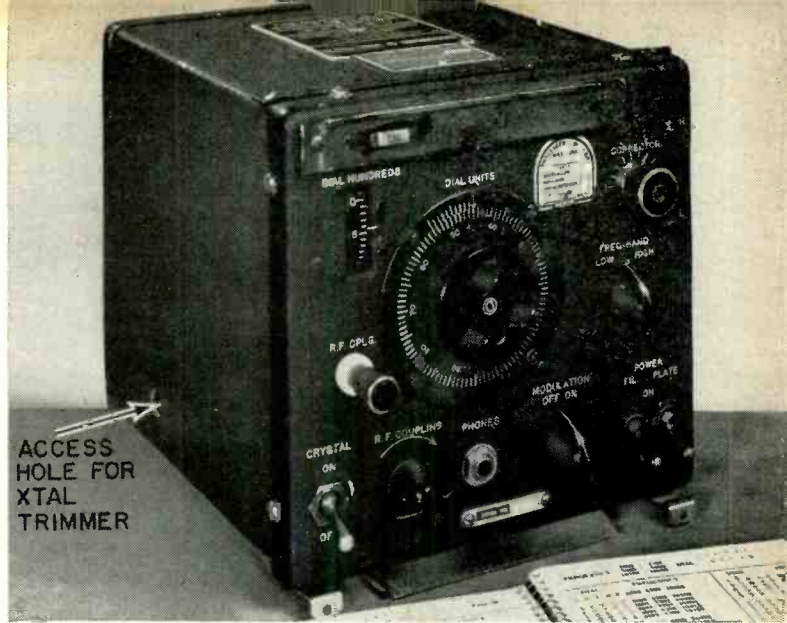
The only thing different about modified LM is small hole in side to provide access to crystal trimmer.
