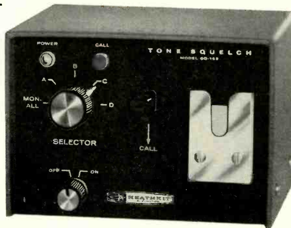
Front view of Heathkit GD-162 Tone Squelch—a selective-calling system and tone-operated squelch.
