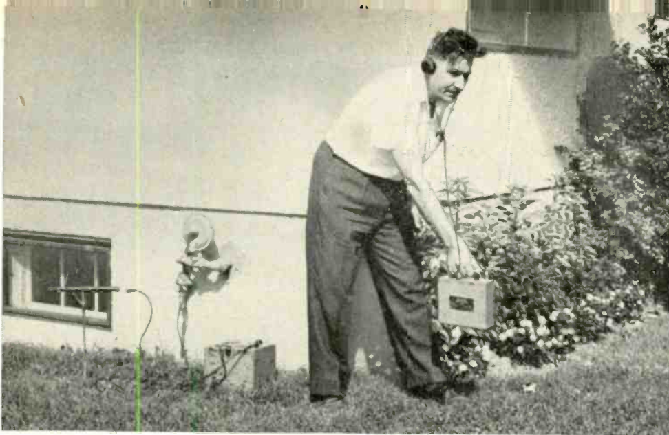
How to trace a shorted cathode, 5000 square feet or more of cathode, that is. Hook up an audio pulse generator to your cathodically protected gas main and a ground probe (left). Then, with the receiver unit, follow the beep-beeps as they take a path to ground through the short.
