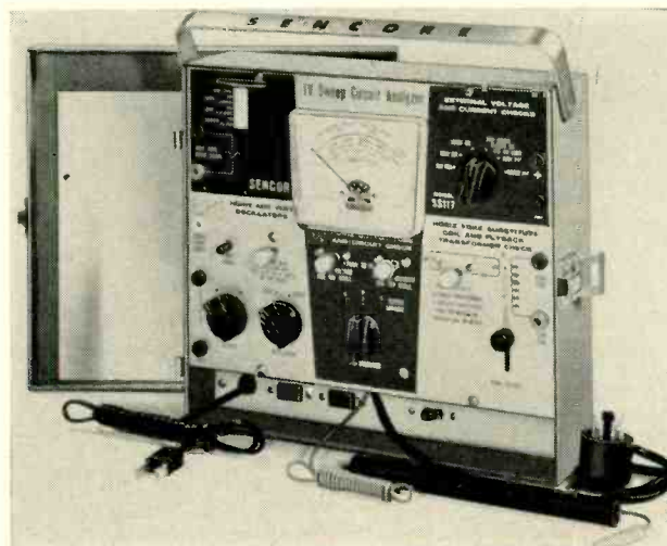
One of the more useful TV service instruments: the Sencore SS117 Sweep Circuit Analyzer.
