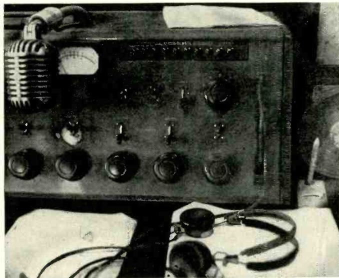
Typical ac-powered remote. Ac power supply at right is on end of long cable to keep hum away from sensitive input transformers.
