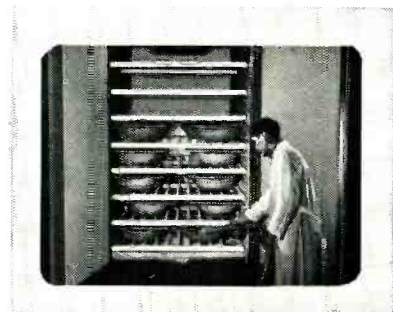
Drying ovens remove moisture from phosphor
