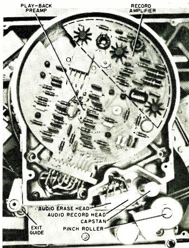
The scan assembly of the recorder with the top cover removed.
