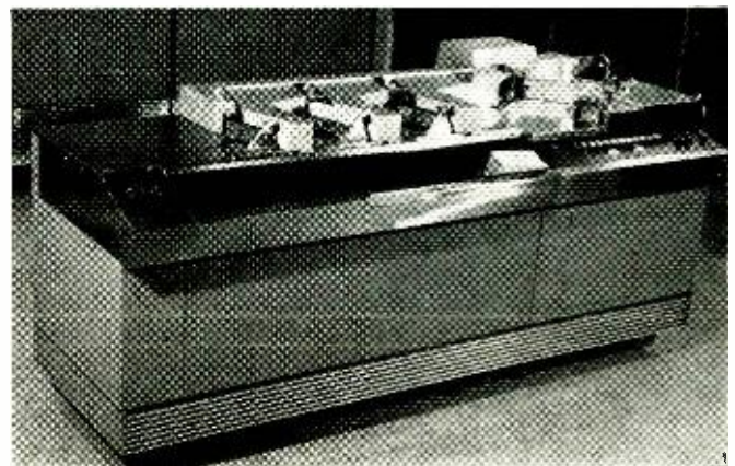
An RCA-developed optical character reader takes advantage of scanning ability of the TV vidicon tube. The device reads data on 90,000 utility bills or insurance premium notices an hour.
