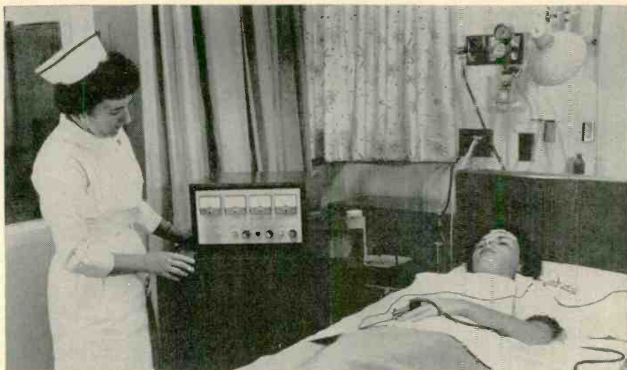
The Executone-Gulton Physiological Monitoring System in use in Perth Amboy General Hospital. The unit shown is measuring systolic and diastolic blood pressure, heartbeat and breathing rate. Readings are given at 30-second intervals on both the portable bedside unit and at a central console.
