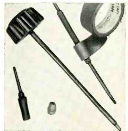
Fig. 5—Alignment tools are much easier to use if you build up their diameters or add knobs. Rubber erasers and plastic tape are useful here.
