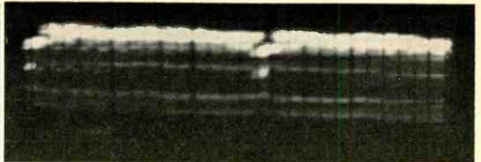
Fig. 5—Whites almost totally compressed. Screen went blank.
