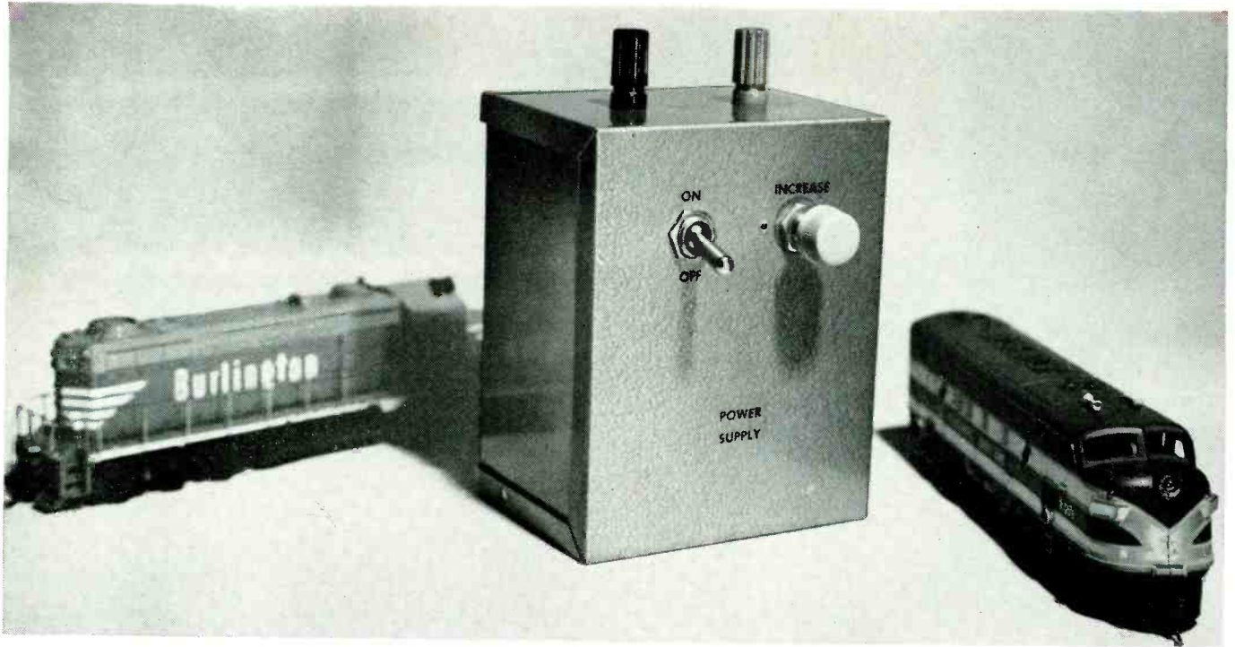
The versatile semiconductor version of a thyatron makes simple battery charger, slave photoflash, model train control
