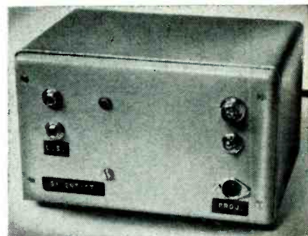
Sole "operating control" on front panel is on-off switch. Operation is completely automatic.
