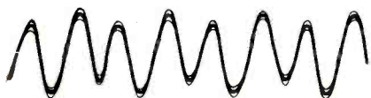
Fig. 6—Unsynchronized 38-kc signal wobbles and flutters erratically, like this. It should be adjusted to look like Fig. 5.
