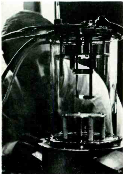
Dr. Foster and the vacuum-deposition equipment used in producing evaporated-layer ultrasonic transducers.
