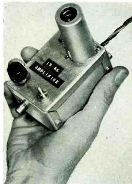
Tiny 19-kc amplifier can be fastened on chassis or case of FM tuner used for test purposes.
