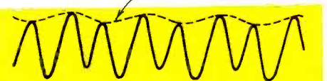
Fig. 5—38-kc voltage at input to demodulating diodes may look like this. Residual 19-kc signal is common and usually harmless.
