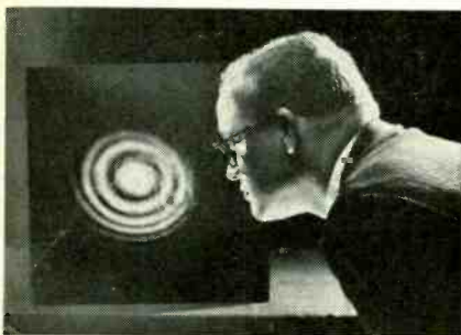
Inventor Louis Enloe examines the interference rings produced by two laser beams being transmitted at exactly the same frequency and with a constant phase difference.
