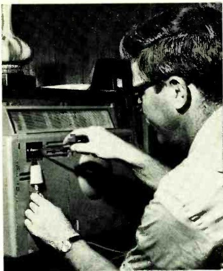
Fig. 4—Set-mounted matching transformer (also a balun) matches 75-ohm coax to 300-ohm set input.
