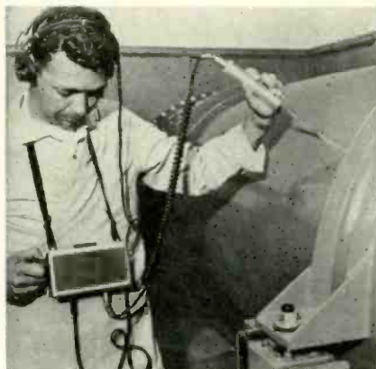
Engineer checks for point of greatest noise in 2-mev flash X-ray system.
