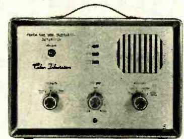
RCA WR-64B Color Bar/Dot/Crosshatch Generator
