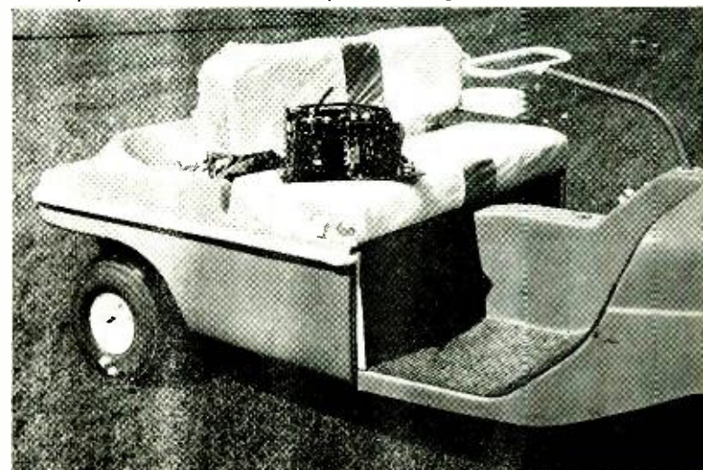
This golf cart employs SCR's for speed control. The entire electronic package with the throttle rod coming out of the top of it has been removed and placed on the golf-cart seat.
