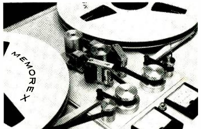
Close-up view of the closed-loop tape drive system used.
