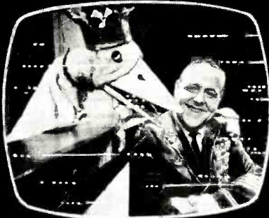
Coaxial Cable Ignition noise minimized—but not eliminated.
