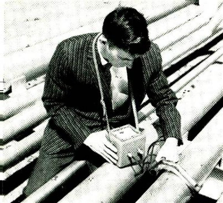
Fig. 7. Portable gamma-ray thickness gage checks pipe walls.
