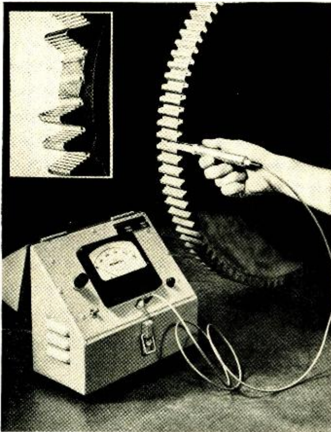
Fig. 6. Test probe locates cracks in a non-magnetic gear.
