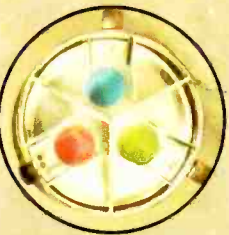
Conventional RCA Color-Tube Gun
