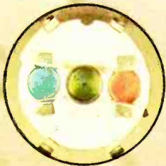
New G-E In-Line Color-Tube Gun
