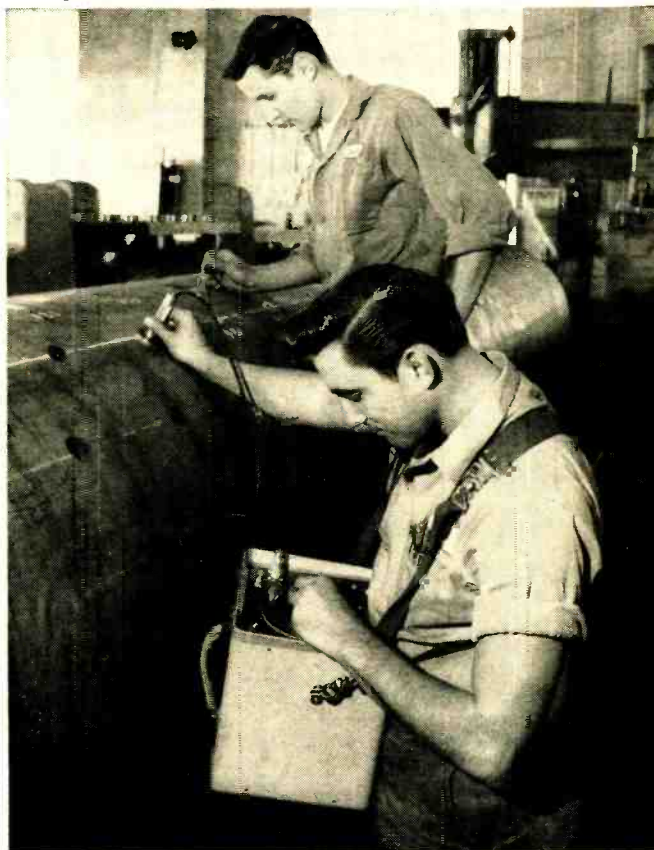
Fig. 5. Portable ultrasonic thickness gage in use. Note the grease couplers placed at the desired pipe testing locations.
