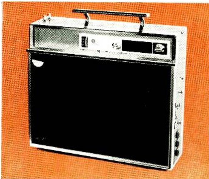
Fig. 1. Exterior (left) and interior (right) of the Westinghouse 19-inch transistor TV set. According to the manufacturer, the black glass reduces glare and improves contrast.
