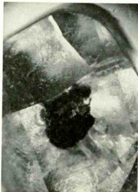
Left: a diamond die pierced by the laser beam before polishing; right, how the die appears after being polished and finished by conventional methods.
