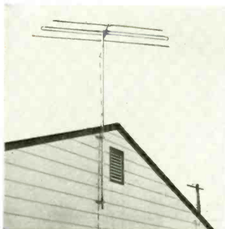
Outdoor antenna is in the clear, picks up more signal than interference.
