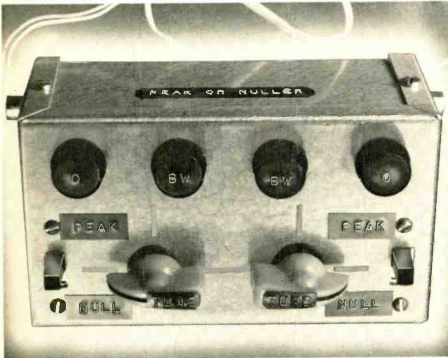
Front view of the completed twin Q multiplier (Peak or Nuller) receiver accessory.
