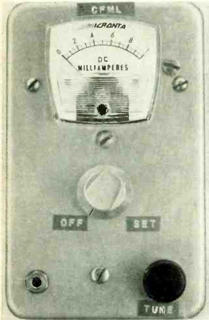
Fig. 5—A meter and only two controls is an indication of the locator's simplicity and ease of operation. The jack at lower left is for the audible monitor.
