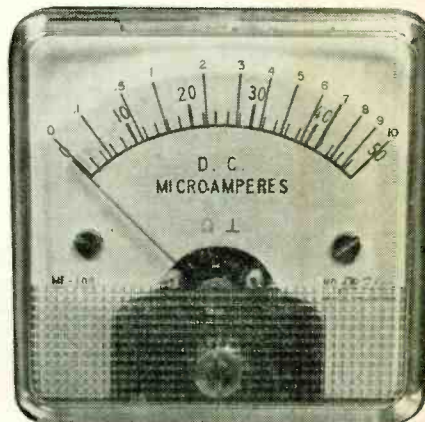
As you calibrate the meter with a known rf signal, mark the meter face by hand.
