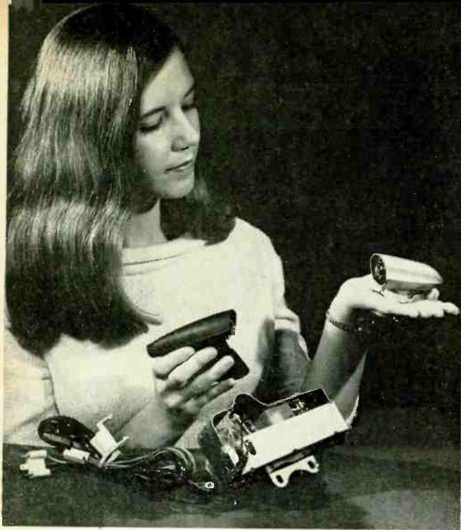
GM's Guide-Matic solid-state headlight dimmer (right) replaces vacuum-tube unit.
