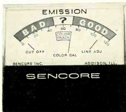
Fig. 3—Central portion of meter is calibrated to read out maximum permissible tracking variation, to predict ability to obtain proper highlights and gray scale.
