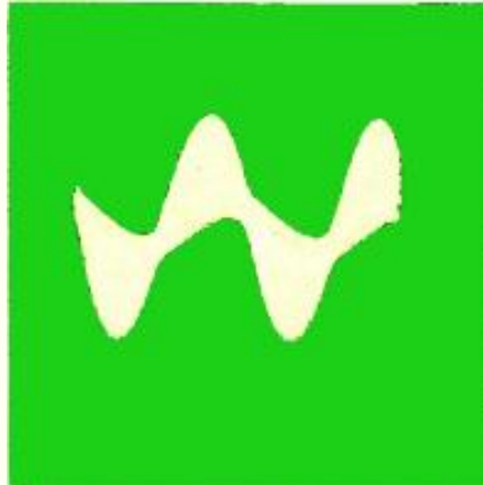
Fig. 4—Severe phase distortion of recovered composite signal at FM detector caused by misalignment of i.f. circuits. This results in tremendously reduced channel separation.
