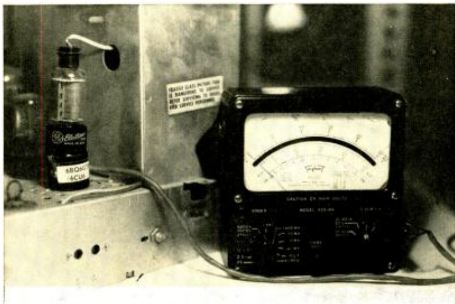
Home-made cathode-current adapter in use. See Fig. 2 for construction. Tab on left side of base goes to grid pin. You can check grid drive from above the chassis.
