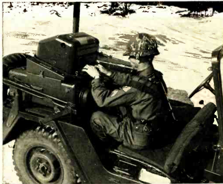
This corporal is teletyping a message via a 400-watt FSK/SSB system that operates on any rtty channel from 2 to 30 MHz.
