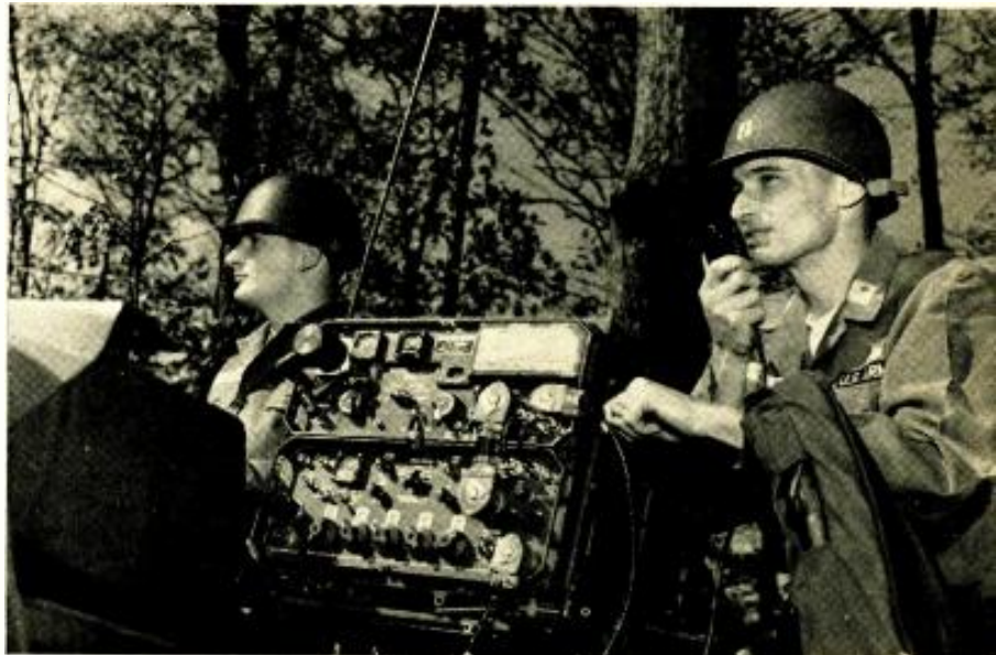
This AN/GRC-106 single-sideband communications system is complex and requires trained operators and repair men. Specialists receive tops in pay.
