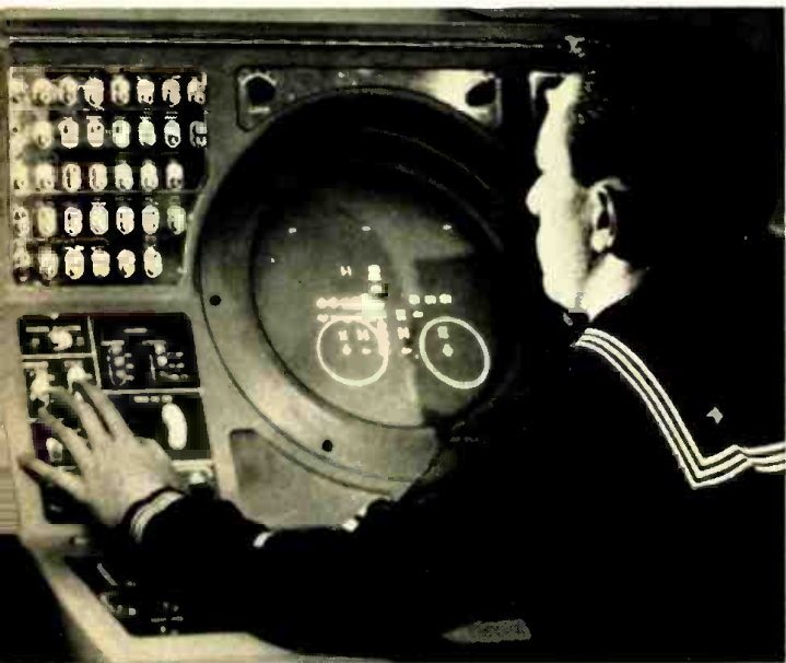
Navy's Tactical Data System displays aerial, sea-surface and submarine targets. Developed by Hughes, it is kept up by Navy.
