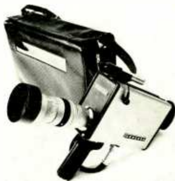
CONCORD'S VTR-400 (inside case) uses 1/2-inch tape running at 12 ips. It has two rotary heads on both record and playback, and has 14-min recording time.
