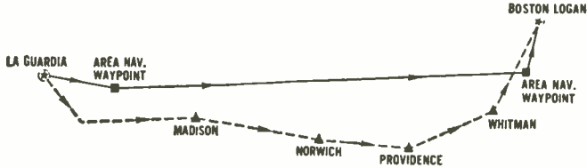
Area navigation vs. conventional navigation (dashed line) from New York to Boston. Below, the display chart and (left to right) autopilot controller, distance/time display, computer control and computer.
