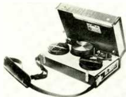
TRIPOD ARRANGEMENT in Sony's vtr camera (above) provides stable base for some shots. Panasonic's NV-3080 (left) weighs only 21 pounds with its camera and batteries, and uses 1/2-inch tape.
