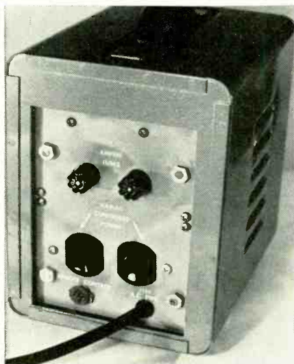
REAR PANEL VIEW shows duplex receptacles, remote jack J8 and fuses. Remote control can be safety feature.
