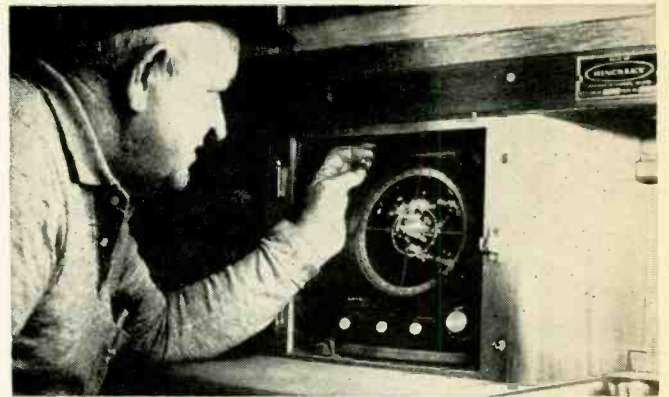
SMALLER THAN A BREAD BOX , Raytheon’s Model 2900 radar fits into the limited space found on most pleasure boats. The transistorized radar paints an electronic picture of land contours and other vessels up to 32 miles away. Its 33-1/2 inch radome-protected antenna weighs only 48 pounds. The radar is offered by Raytheon Marine Products, at $2,850. ★
