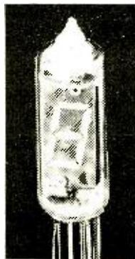
Fluorescent vacuum readouts. These readouts consume low power, and have a highly visible blue green display. Operates from 25 volts D.C., and 1.5 volts at 42 milliamps for filament. Compatible with 7448 decoder-driver, a most unusual and effective display.
