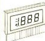
Need a low power display? These liquid crystal displays require less than 1 microwatt per segment. Unlike other liquid crystal displays, these have fast turn on and turn off times, can be time multiplexed, will operate from low voltage AC or DC, can be seen in low ambient lighting, and are TTL compatible. Digits are 0.4" high and each has a decimal pt. LCR 3.5 has "+" and "-" sign and an overflow arrow. Supplied with three connector, specs & app. notes.
