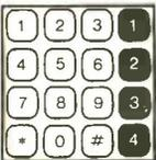
These low cost keyboards are great for home built computers, calculators, touch tone networks etc. Each contact is rated at 40 mA and 25 V. Will interface directly with TTL, DTL, and RTL logic. Employ elastomeric principle for almost infinite life. These come directly from the manufacturer and we supply applications information. Measure 3" on a side and 1/2" deep.
