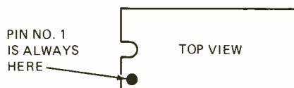
FIG. 1—FINDING PIN 1 of a dual-inline-package (DIP) IC is easy. Just look for the notch in one end as shown here.
