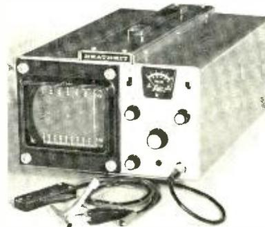
condenser or transistor problems. Features built-in tachometer with 0-1,000 and 0-5,000 ranges, for making carburetor adjustments. No need to adjust sweep width for changes in rpm—simply set it once and special circuitry holds it constant. Front panel controls for four patterns—primary
