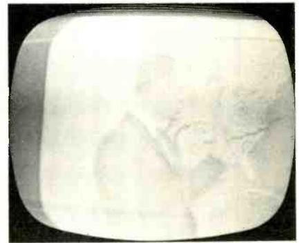
**WASHED OUT—TOO MUCH AGC VOLTAGE.** Rf and i.f. amplifiers are tending to cut off.
