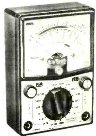
strument measures 5" x 3-½" x 1-¾", is battery-powered, has built-in battery check and all controls and jacks are on the front panel. Comes in a simulated leather carrying case. \$54.95.—**Mura**, 50 S. Service Rd., Jericho, NY 11753.
