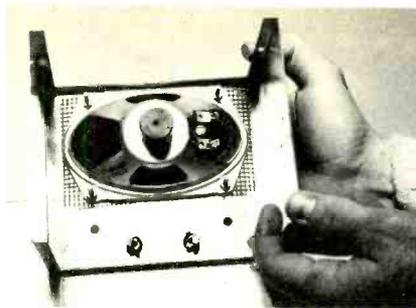
FIG. 5—HOW SPEAKER AND GRILLE are mounted on the front-panel section of the box.
