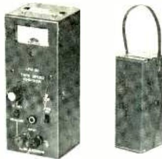
using a 3-kHz tape calibrated for 3-3/4 ips and then using the same tape as a 6-kHz test source for 7 1/2 ips. Test range  $-3\%$  to  $+3\%$ . Input level 100 mV to 10 Vrms. Input impedance 150K.
