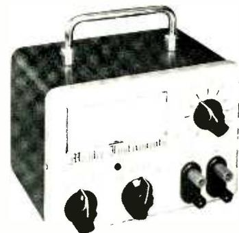
into 600 ohms and 10 mV into 250 ohms. The instrument can be used as an audio voltmeter with 400K input impedance and fullscale ranges of 1 mV to 100 Vrms in eleven 10-dB steps. Frequency response (-6-dB points) is 0.3 Hz to 100 kHz. The -10 to +2-dB scale is referenced to 1 mW into 600 ohms. Powered by eight "C" cells.
