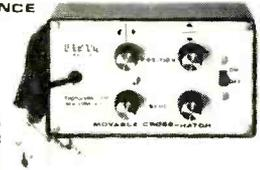
THE GENERATOR IS A TV TRANSMITTER GENERATING ONE VERTICAL AND ONE HORIZONTAL LINE EACH MOVABLE OVER THE TV SCREEN OUTPUT. CONNECTS DIRECTLY TO SET ANTENNA ONLY 3 1/2 x 6 x 2" IDEAL FOR CARRYING IN TOOL CADDY. KIT IS COMPLETE WITH ALL PARTS, DIAGRAMS AND INSTRUCTIONS.
