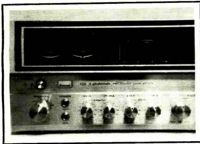
FIG. 2 — LEFT SECTION OF FRONT PANEL includes meters, speaker selector, two phone jacks, and two sets of tone controls.
