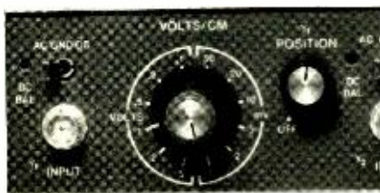
FIG. 1—A CLOSEUP PHOTOGRAPH of the vertical input of a Heath IO-4510 dual-trace 15-MHz oscilloscope. Notice the three position input coupling switch, with the center position marked ground.
