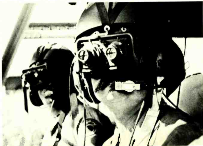
FIRE-FIGHTING HELICOPTER PILOTS of Los Angeles County wear these bifocal light-amplifying goggles that permit them to see at night while flying over dangerous mountain terrain to fight forest fires, while at the same time keeping an eye on the cockpit instruments.
