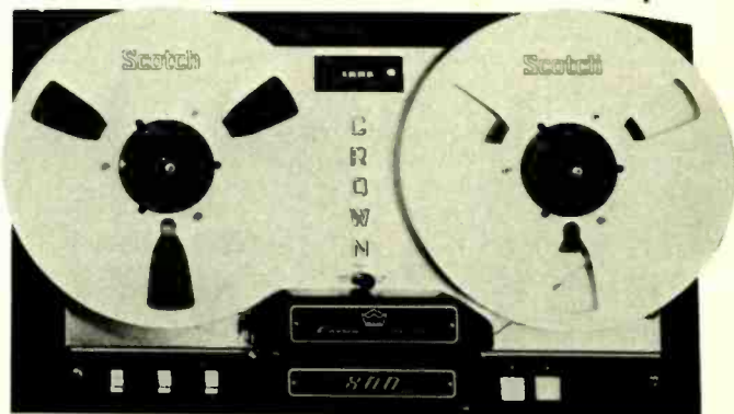
TRANSPORT SECTION of Crown series 800 tape recorders. Audio electronics is a separate circuit.
