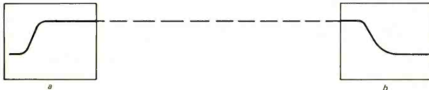
FIG. 15—EFFECT OF TRIGGERING on positive edge is shown in a, while negative edge is shown in b.
