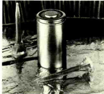
NEW HIGH CAPACITY/DISCHARGE CELL developed by General Electric offers 20 per cent improvement in deliverable capacity over older sub-C nickel-cadmium cells. Capacity is 1.2 amp-hrs at 1.2 volts. It measures 1.6 inches high with a .875-in. diameter.
