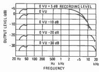
FIG. 3—RECORD/PLAYBACK frequency response of cassette tape.
