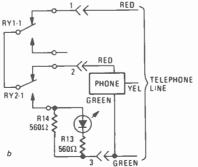
FIG. 7—TELEPHONE CONNECTIONS. Use the connection (a or b) that makes terminal 1 positive, or the one that causes dialing indicator to light when dialing.
