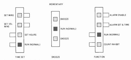
FIG. 8—SWITCH FUNCTIONS of the three slide switches.
