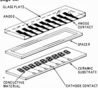
THIS GAS-DISCHARGE DISPLAY is a part of a digital clock you'll want to build. For details turn to page 67.
