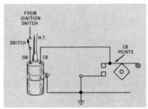
FIG. 2—IGNITION IMMOBILIZER operates by disabiling vehicle's ignition circuit.
