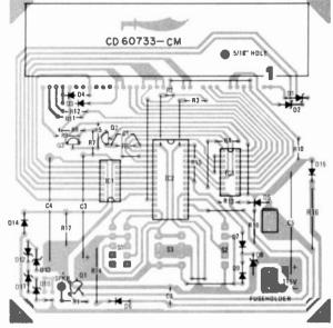
FIG. 6-FOIL PATTERN of PC board shown half-size.
