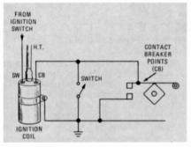
FIG. 1—IMMOBILIZER operates by shorting contact breaker points.
