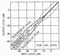
FIG. 8—INPUT/OUTPUT characteristics of the Super-ANRS circuit.
