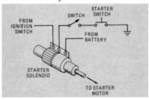
FIG. 3—STARTER IMMOBILIZER operates by opening starter-motor circuit.
