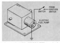
FIG. 4—FUEL-PUMP IMMOBILIZER operates by opening electric fuel-pump circuit.
