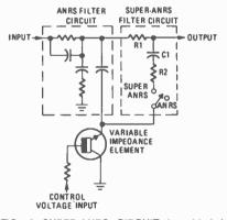
FIG. 4—SUPER-ANRS CIRCUIT is added to basic ANRS circuit and is controlled by a variable impedance.
