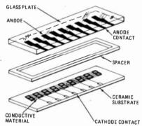
FIG. 1-CONSTRUCTION of the gas-discharge planar display. Like segments of each digit are connected together for multiplexed operation.
