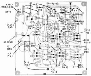
FIG. 5-COMPONENT LAYOUT of Board A
