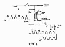
all-tube set. Note the heater circuits. There are two of them in parallel, both of which are fed through diode D6. The heater voltage is given as -55 volts, so it is evidently read on a DC voltmeter! A standard AC voltmeter would probably give you a very weird reading since it's calibrated for sinewayes.
