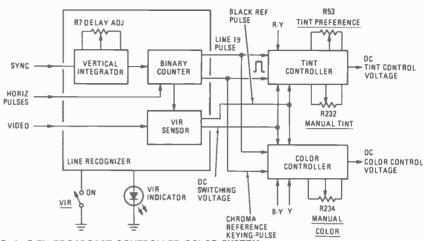
FIG. 4-G-E's BROADCAST CONTROLLED COLOR SYSTEM.
