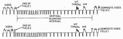
FIG. 1-RELATIVE POSITION OF VIR SIGNAL in the composite video signal.
