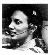
that it can be close to the lips and moved aside when not in use. The push-to-talk switch has a clip for convenient attachment to a shirt or blouse.
