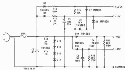
FIG. 5—POWER SUPPLY has split high-voltage supply to drive display and low-voltage source for IC's. Timebase is derived from low-voltage supply.
