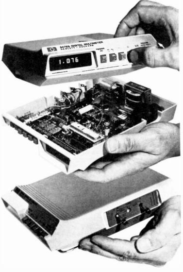
Five functions—all the functions you want and need in a low-cost DMM. Simply push the appropriate button to read AC volts, DC volts, AC or DC current, and ohms. There's no worry about polarity or zero... they're both automatic.
