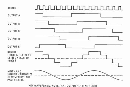
AN EIGHT-STEP GENERATOR, as used in a digital cassette recording system.
