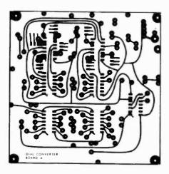
FIG. 3 (left)—PRINTED CIR-CUIT pattern for Board-A shown half-size.
