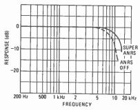
FIG. 10—RECORD/PLAYBACK frequency response with and without Super-ANRS.
