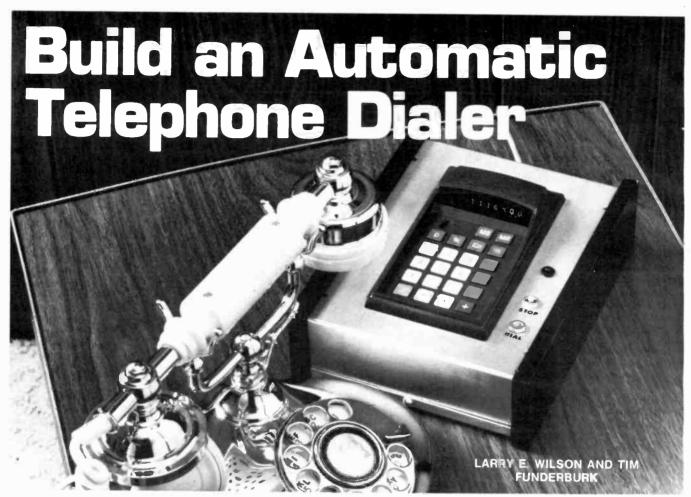
Convert an ordinary calculator into an automatic telephone dialer. If the calculator has a memory, you can store a telephone number as well. And when not dialing, the unit can be used as an ordinary calculator
