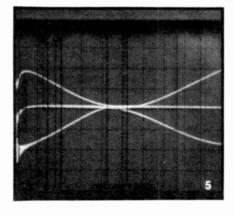
posed for reference. High and low filter response corresponds exactly to manufacturer's claims, with the rumble filter exhibiting a 6 dB-per-octave slope and the high-cut filter attenuating frequencies above about 5 kHz at a rate of 12 dB-per-octave.
