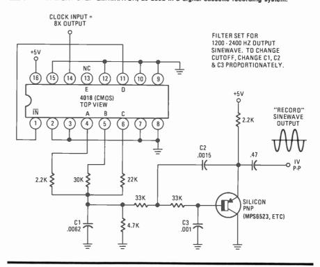
10-STEP SINEWAVE GENERATOR drives the transmitter speaker of a MODEM.
