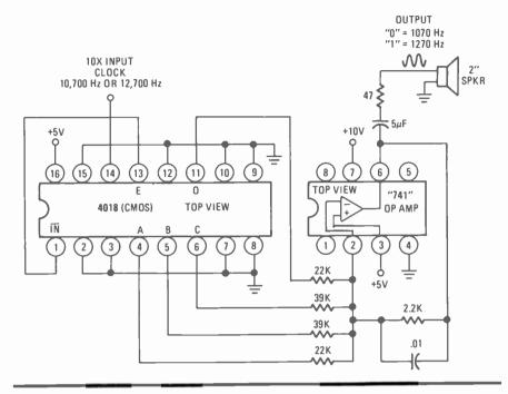
THREE-STAGE DIGITAL SINEWAVE GENERATOR. Resistance values are shown in ratios (parentheses) and ohms. The amplitude of the harmonics are also shown.
