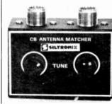
band. Most transceivers operate into 50-ohm loads, delivering maximum power with minimum distortion and harmonic radiation. A mismatch between antenna and transceiver occurs because the antenna impedance varies widely with frequency and physical location. The Antenna Matcher assures that the transceiver will be matched to the antenna at any time and on any channel with minimum harmonic radiation. Matches radio to antenna impedances of 35 to 150 ohms. Fitted with SO-239 connectors
