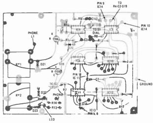
FIG. 6-COMPONENT LAYOUT of Board B.
