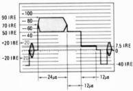
THE VIR SIGNAL makes color TV pictures perfect. It's tucked away on line 19 between two horizontal sync pulses. See how it works on page 83.
