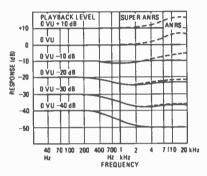
FIG. 6—PLAYBACK CHARACTERISTICS of the ANRS and Super-ANRS circuits.
