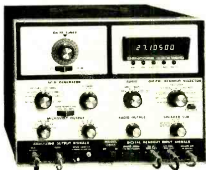
FIG. 4—SENCORE MODEL CB42 contains several instruments that are needed to service CB gear, plus extra features some systems do not have. With this setup, few other instruments are needed on the bench.
