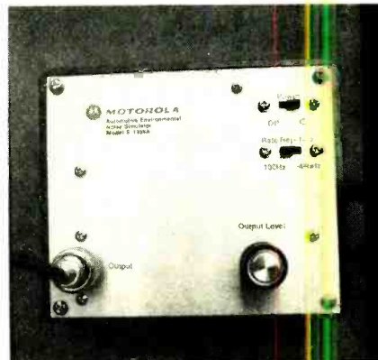
MOTOROLA NOISE SIMULATOR generates bursts of pulses that resemble actual ignition interference.
