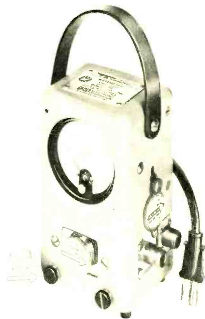
BIRD MODEL 43 wattmeter has long been a standard in communications servicing. Newer model 4314 is peak-reading version for SSB.
