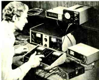
FIG. 2—TEST INSTRUMENTS from B&K/Precision have their own interconnect panel—a special instrument that automatically switches over from receive to transmit.
