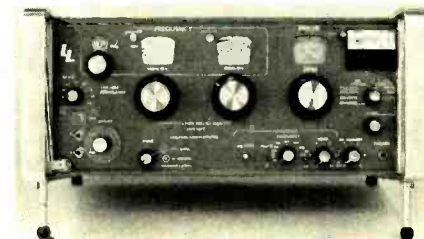
FIG. 5—LAMPKIN LABORATORIES has been manufacturing frequency meters since the early days of communications. The model 107C is highly accurate for AM and FM servicing.
