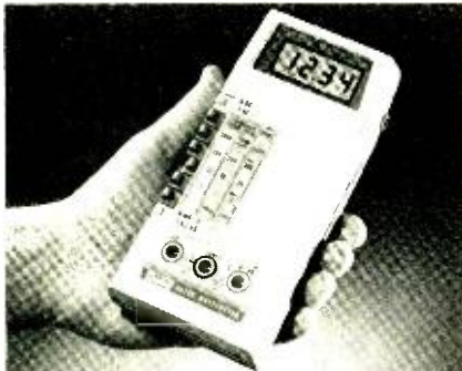
HANDHELD DIGITAL MULTIMETER, Fluke model 8020A features liquid-crystal display, common in watches but not in test gear. Cuts battery drain. Range switches are along one side.
