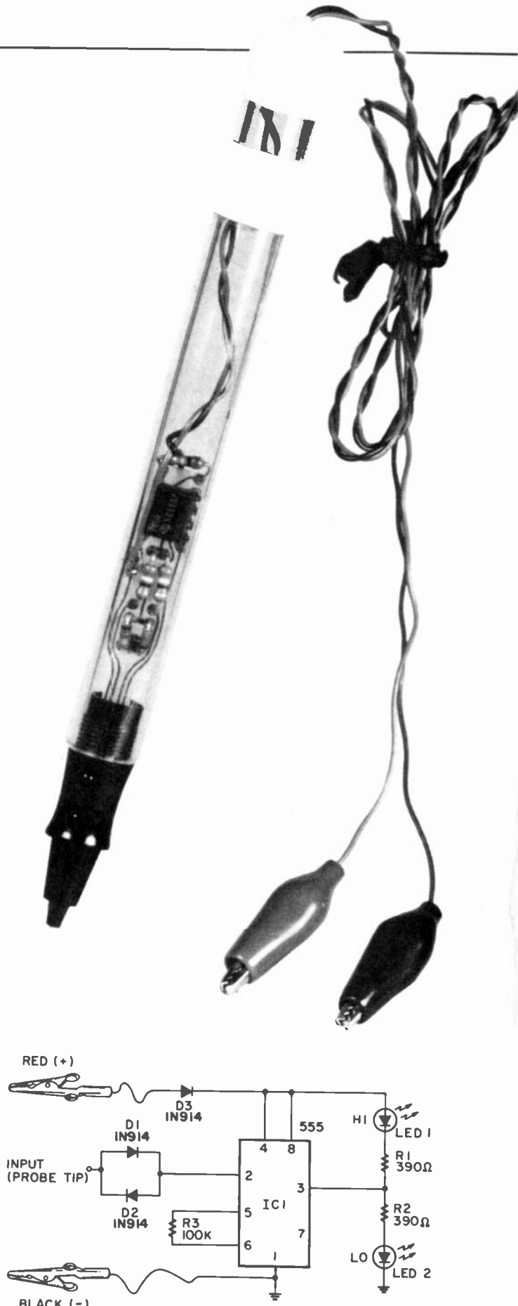
FIG. 1—SCHEMATIC DIAGRAM of the logic probe. Device can be powered by 3.5 to 15 volts tapped off the supply in the device under test.
