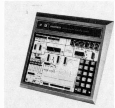
FIG. 5—A BUILT-IN solderless breadboard is among the features of the ET-3400 computer trainer from Heath.
