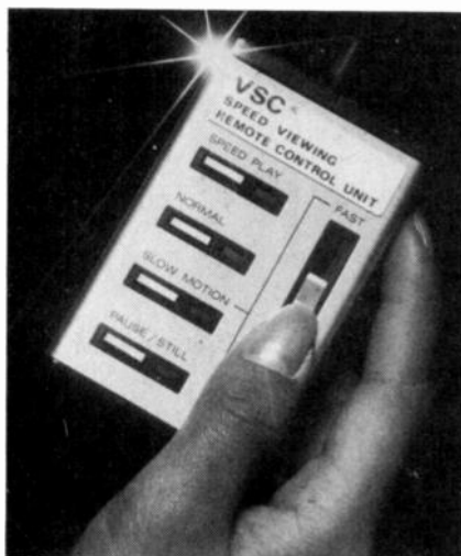
SPECIAL SPEED-VIEWING CIRCUITRY permits viewer to listen to sound while he scans the tape. The circuitry is in the VCR.
