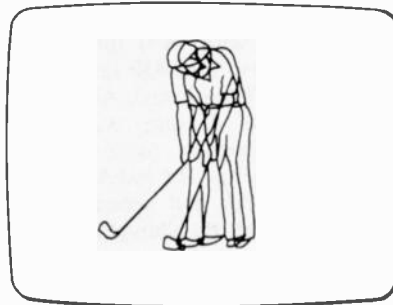
FIG. 2—THIS BLURRED PICTURE was caused when the two fields shown in Fig. 1 were combined to form this stop-frame picture.
