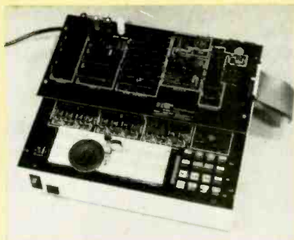
FIG. 1—MINI-MICRO DESIGNER, the MMD-1, from E&L Instruments, is shown with its memory expansion board.
