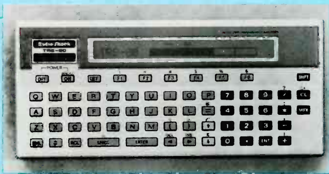
FIG. 2—AMONG THE FEATURES of the new TRS-80 model PC-2 is a new, more powerful version of pocket BASIC.
