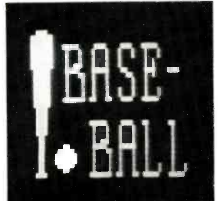
FIG. 11—NOTE HOW TITLER can combine alphanumeric and graphics in one display.
