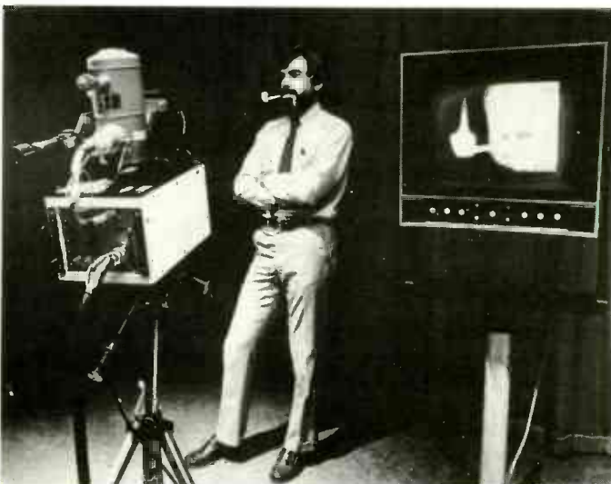
THIS CAMERA TAKES PICTURES WITH HEAT WAVES, much as an ordinary television camera does with light waves. Warm objects like scientist Gary Hughes' skin and lighted pipe show up white, while the mustache shows dark spots.
