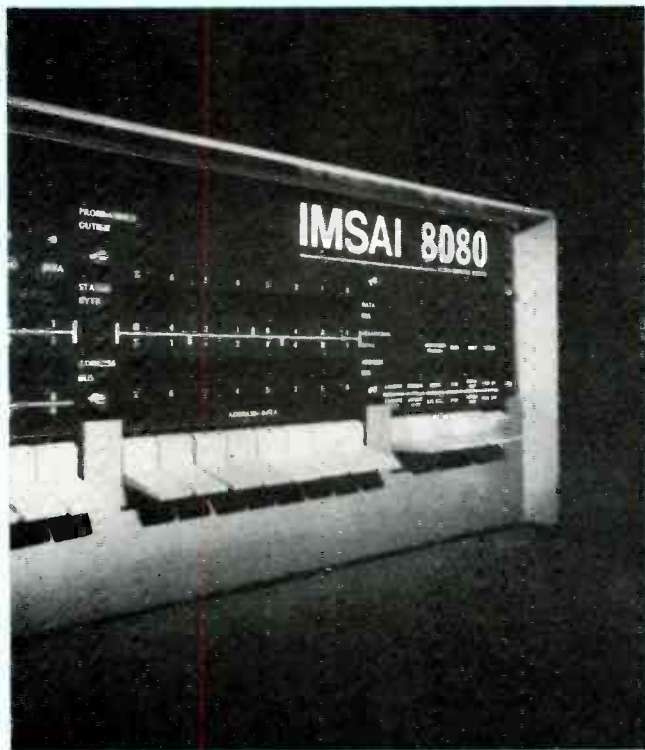
FIG. 1—AN EARLY PERSONAL COMPUTER, all data had to be entered manually, and in binary form, on this IMSAI computer.
