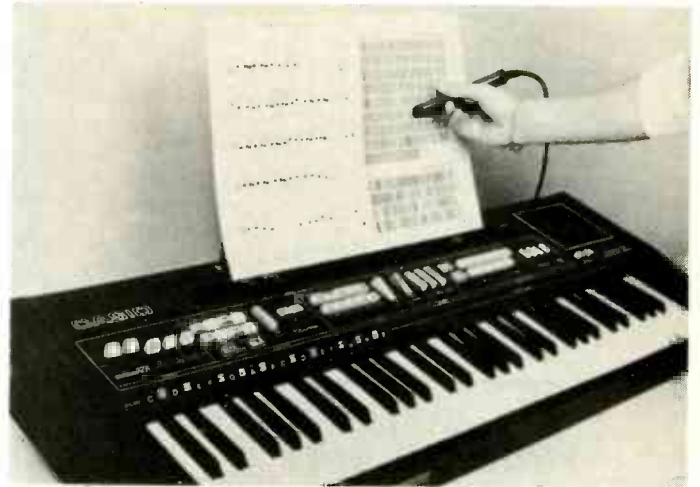
THE CASIO CT-701 player piano records music in its memory from a supermarket-type bar chart, scanned—also in supermarket fashion—with a light pen. It is also a teaching tool, lighting lights over each key the student should press in learning a piece of music.
