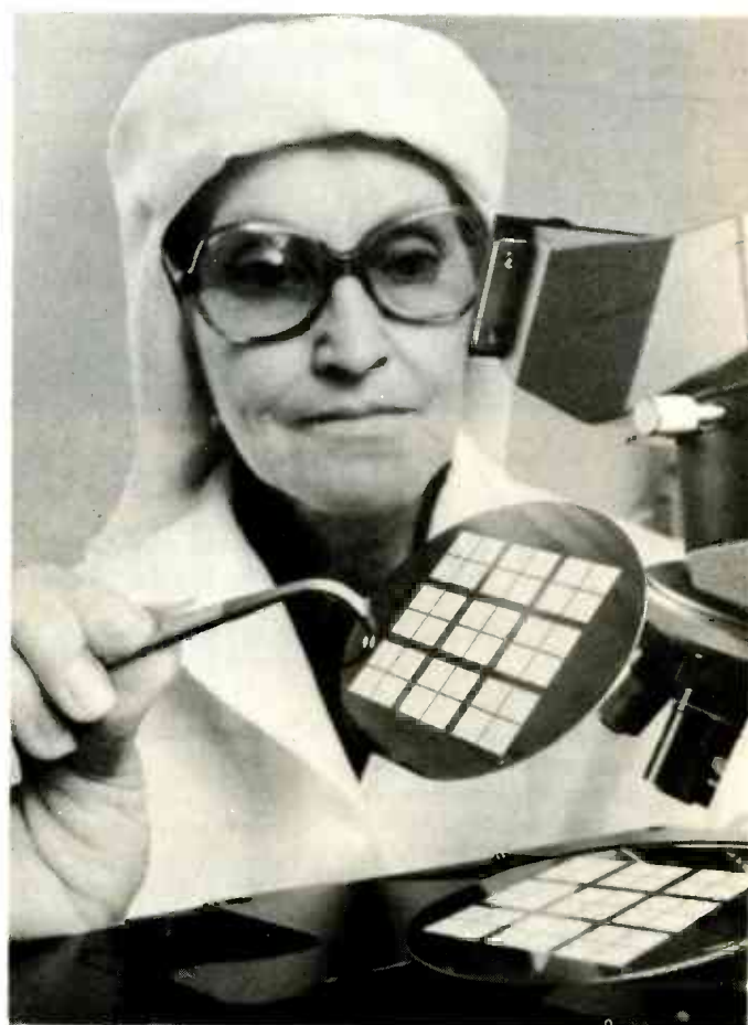
POWER SEMICONDUCTOR CHIPS are being inspected for impurities by GE lab technician Beatrice Hatch. Each of the chips, measuring 0.3-inch square, contains more than 60,000 separate but interconnected circuit elements. This is the first time that VLSI (Very-Large-Scale Integration) techniques have been applied successfully to fabricating such a large-power semiconductor chip.
