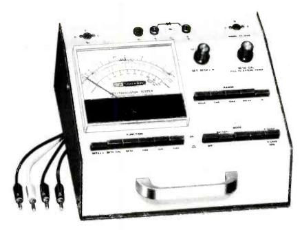
A TRANSISTOR TESTER, such as the one from Heathkit shown here, should be used to check all surplus and salvaged transistors before use.
