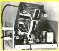
BUILD THIS FREQUENCY MULTIPLIER and increase the low-frequency range and accuracy of your frequency counter. Complete construction details start on page 43.
