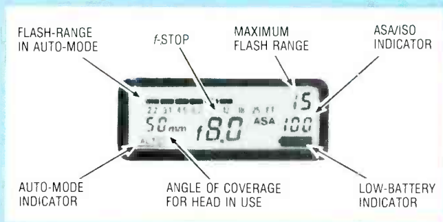
FIG. 3—A CLOSE UP VIEW of the 5600's LCD display shows just how much exposure information it can provide.
