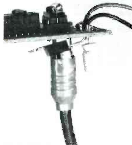
FIG. 4—BEND IC1 OVER BACKWARD on the bottom of the board as shown.
