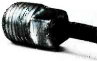
FIG. 7—COMPLETED FILLER-BOLT probe with cable attached.
