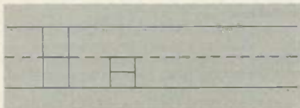
FIG. 3—IN MOST CASES, letter height determines a letter is capitalized or is lower case.
