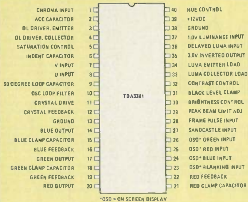
FIG. 10—PINOUT OF THE TDA3301. This Motorola IC contains everything needed to convert luminance and chrominance information into RGB signals.
