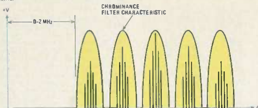
FIG. 6—AN IDEAL CHROMA FILTER would have zero response to about 2 MHz, then comb every 15.734 Hz to 4.5 MHz.
