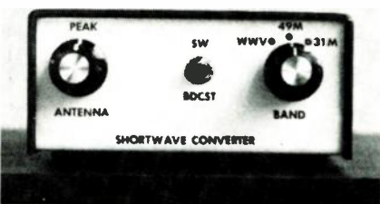
FIG. 7—THE COMPLETED CONVERTER. If you wish, follow the design shown here when laying out your front panel.
