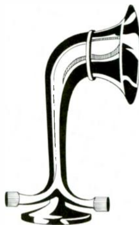
FIG. 9—ONE OF THE EARLIEST ATTEMPTS to get more volume was a small horn that fitted over an earphone.
