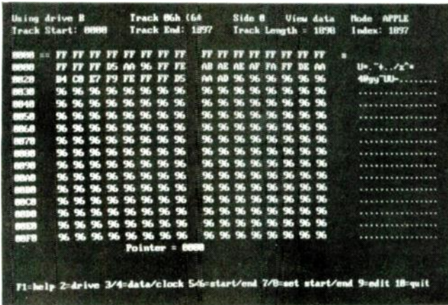
FIG. 3—SECTOR DUMP of an Apple disk (a) and an IBM disk (b).
